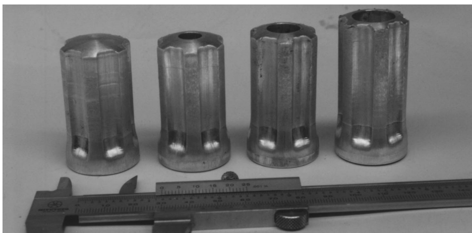
Fig. 13. The hollow billets and the extruded products with different inner radius.
