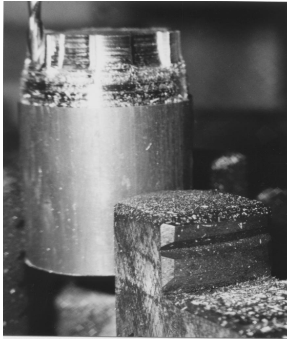
Fig. 12. The finish cutting of the electrode of EDM (with ball-end cutter).
