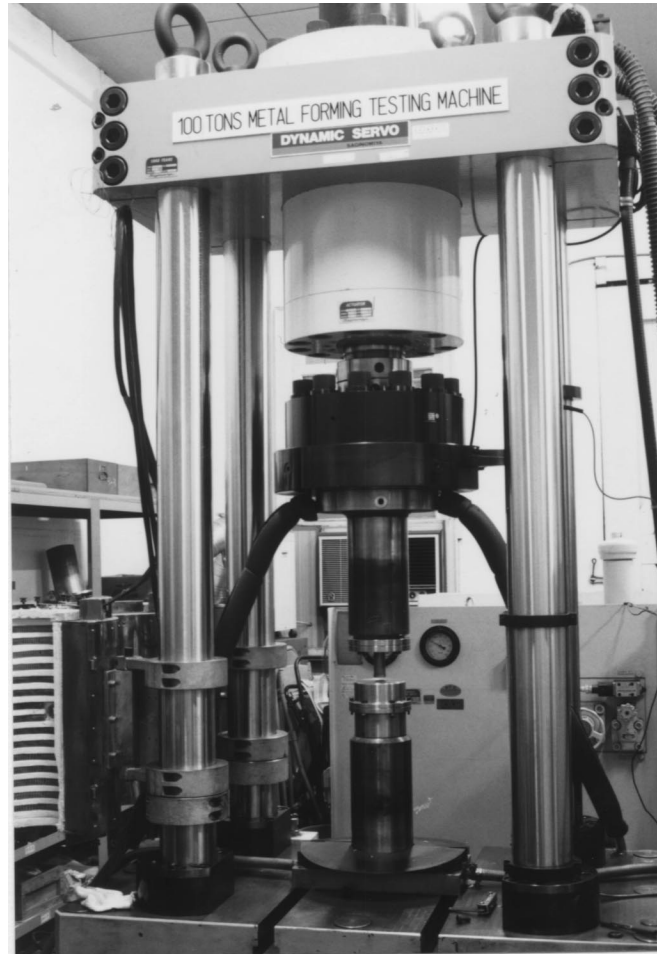
Fig. 6. The Saginomiya 100-ton hydraulic press for compression and extrusion tests.
