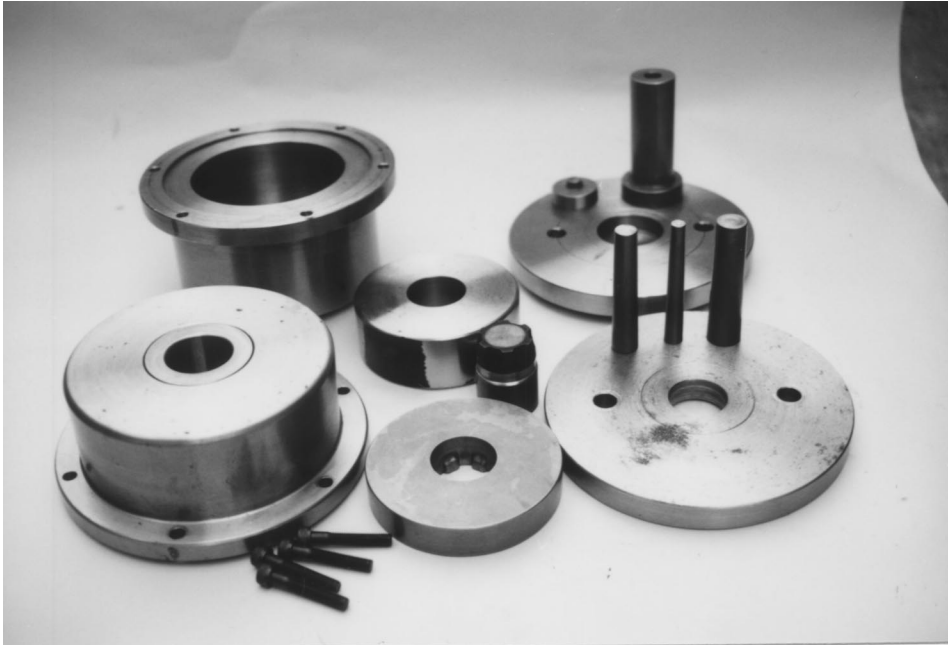
Fig. 7. The components of the extrusion die set (container, ram, mandrels, bolster and die cavity).
