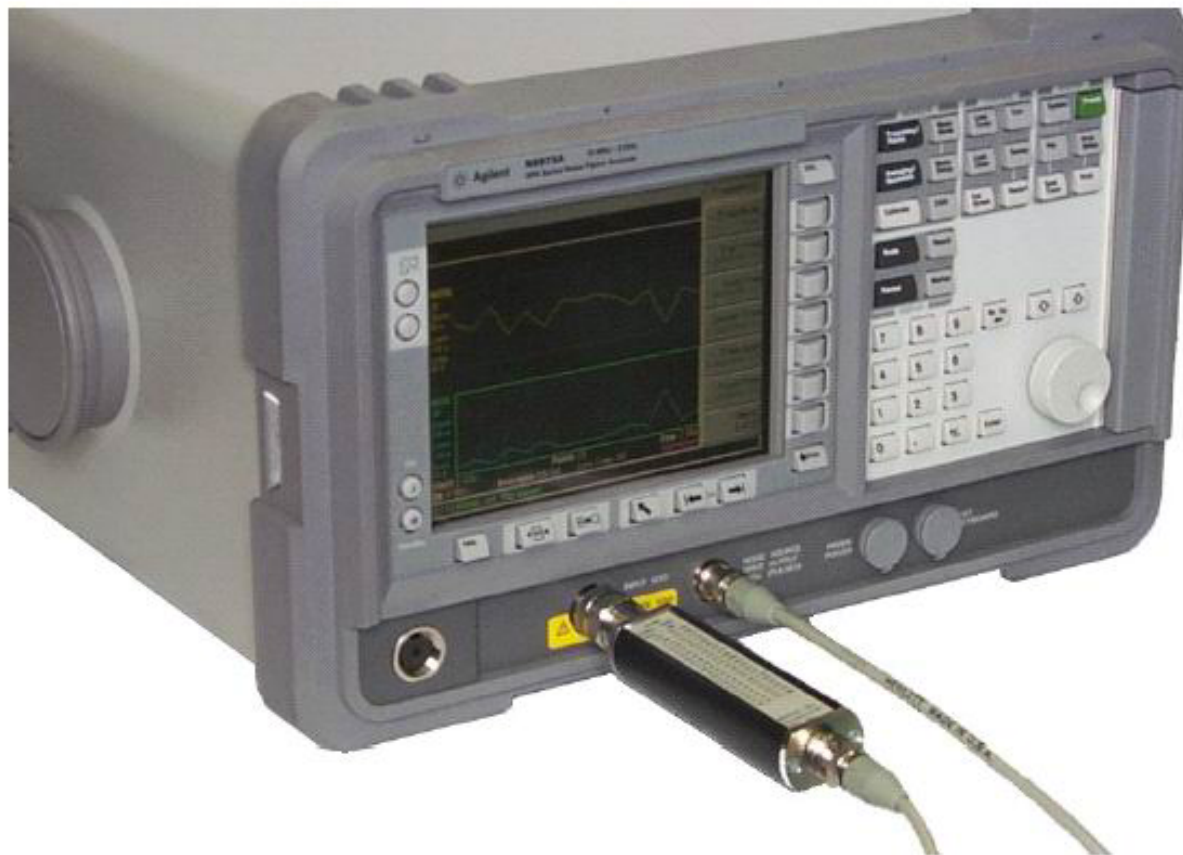
NFA with a Normal Noise Source connected
