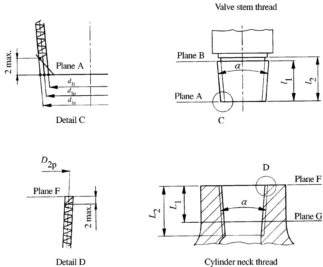
Figure 1: Thread reference planes and diameters
