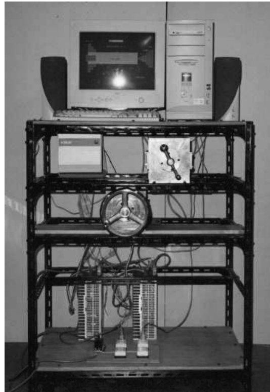
Fig. 1. Learning-training simulator for lathe operations.
