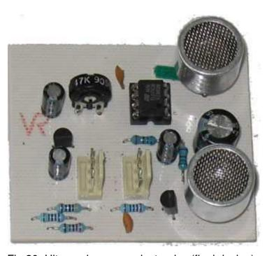
Fig 20: Ultrasonic sensor electronics (final design)
