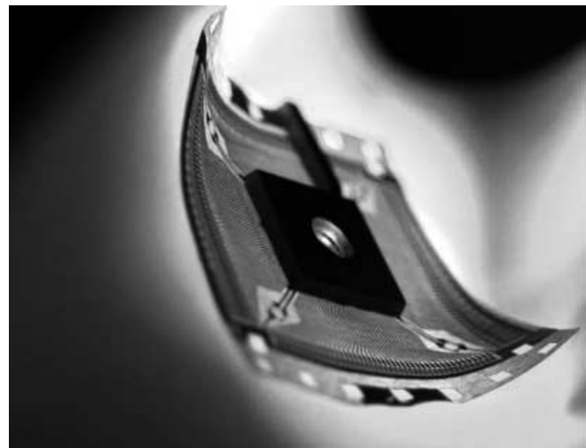
Fig. 2. CavityPack: molding on flex approach to sensor packaging
